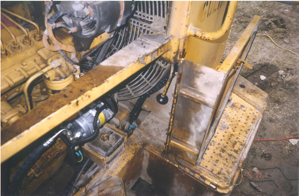
Hoses at compressor and bottom of radiator shroud.
